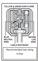
B) Connect the BROWN live wire to the live terminal 'L'.C) Connect the BLUE neutral wire to the neutral terminal 'N'.
